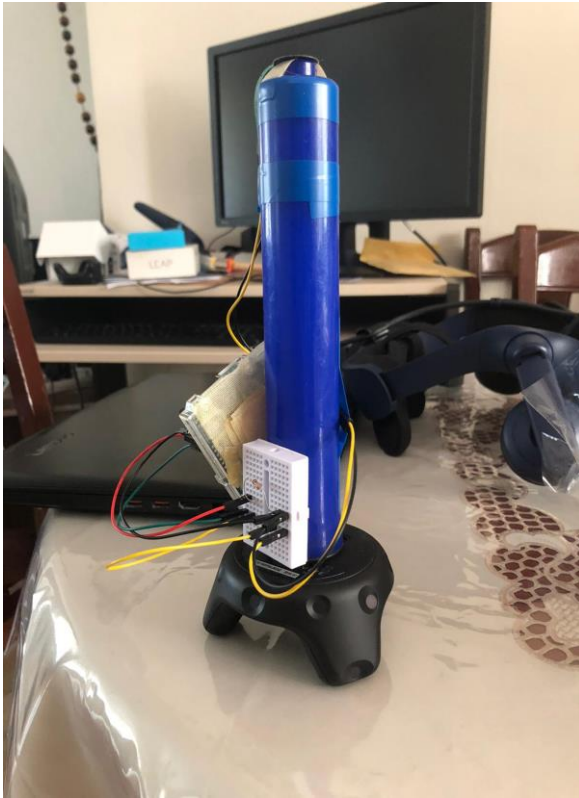
Figure 25 -26: The Arduino setup on the custom made brush
